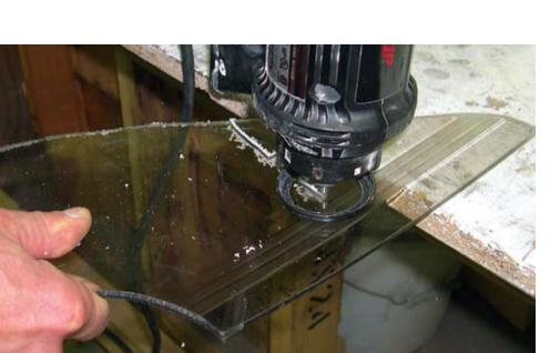
narrow kerf. The tool is not directional and can easily be guided around curves or corners.
